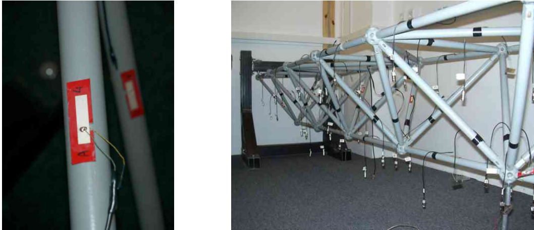
Figure 7: Experimental stand – 3D truss structure. (a) piezo-sensor, (b) general view.
